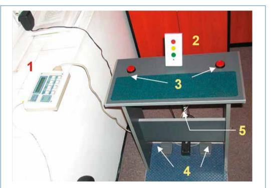
Fig. 1. Device for reaction time measurement MCR - 2001E, 1 – main unit of MCR – 2001 E – microchip meter of reaction time, 2 – semaphore (signaler - releaser of light and sound stimuli), 3 – "manual" manipulators, 4 – "leg" manipulators, 5 – connection system
